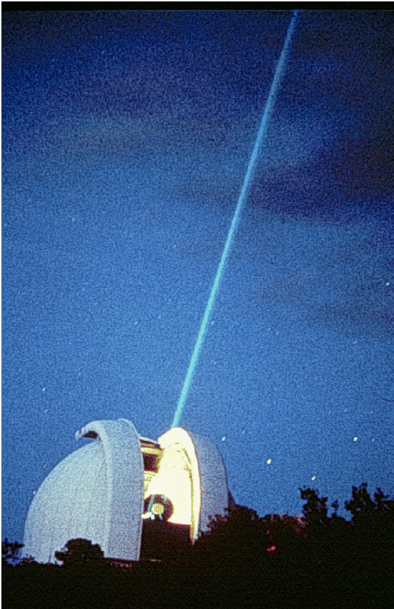
Figure 1. A laser beam sent from an observatory is used to measure accurately the distance between the Earth and the Moon.
